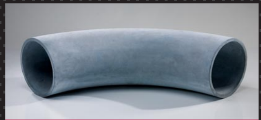
One piece elbow sweep for ash handling. One piece design reduces seams which are often the weak link in severe abrasive wear applications.
