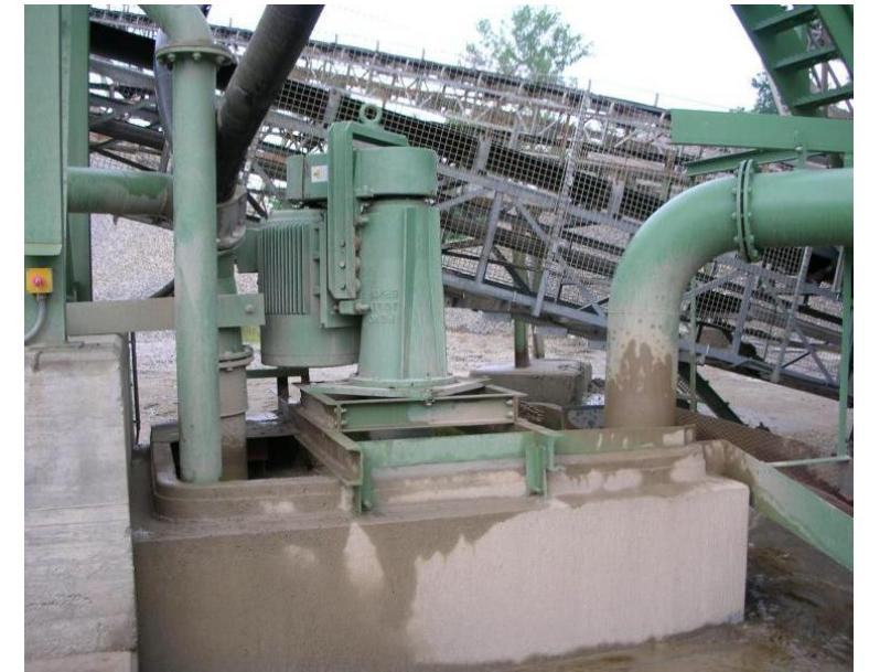
All metal, the PEMO submersible pumps are designed with long life and low maintenance as a priority. The wetted parts of the pump, (volute(s), impeller(s), inlet flange(s), and shaft sleeve(s) are made of an extremely hard iron alloy called, "Hardalloy" which has a hardness rating of over 800 bhn. The hardness of the pump components is the key to reliable performance in rugged applications ranging up to 70% solids, with max size of particles up to 20mm in diameter.
